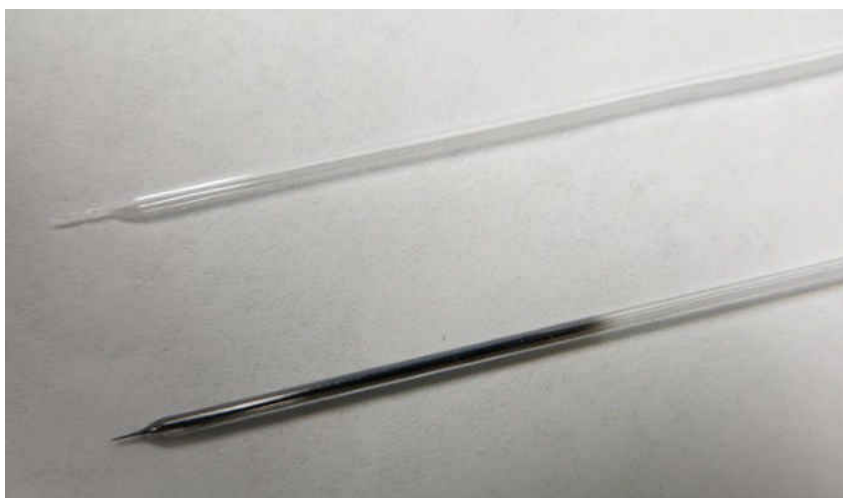
Figure 1: Images of pulled quartz pipette (1.0 mm O.D., 0.5 mm I.D., 10 cm length) before (top) and after (bottom) deposition of carbon.
