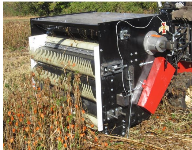
Figure 4.23: Stripping header with guide channels installed
