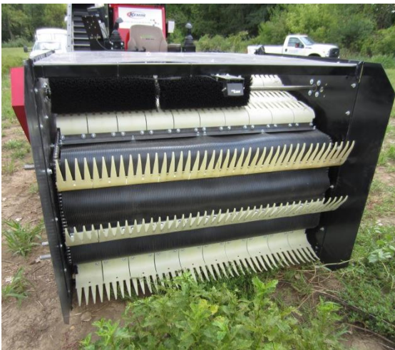
Figure 4.22: Stripping header with cylindrical dislodging brushes. Without guide pin system.
