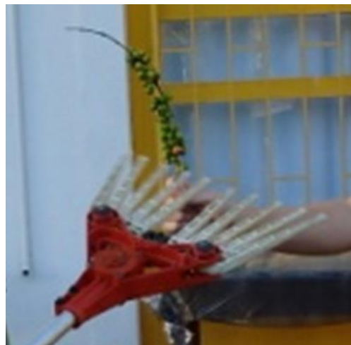
Figure 2.5: PSV end-effector rake fingers
