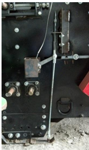
Figure 4.15: Automatic header height sensor and skid assembly
