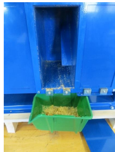
Figure 6.12: Inside of Seedburo tester chamber
