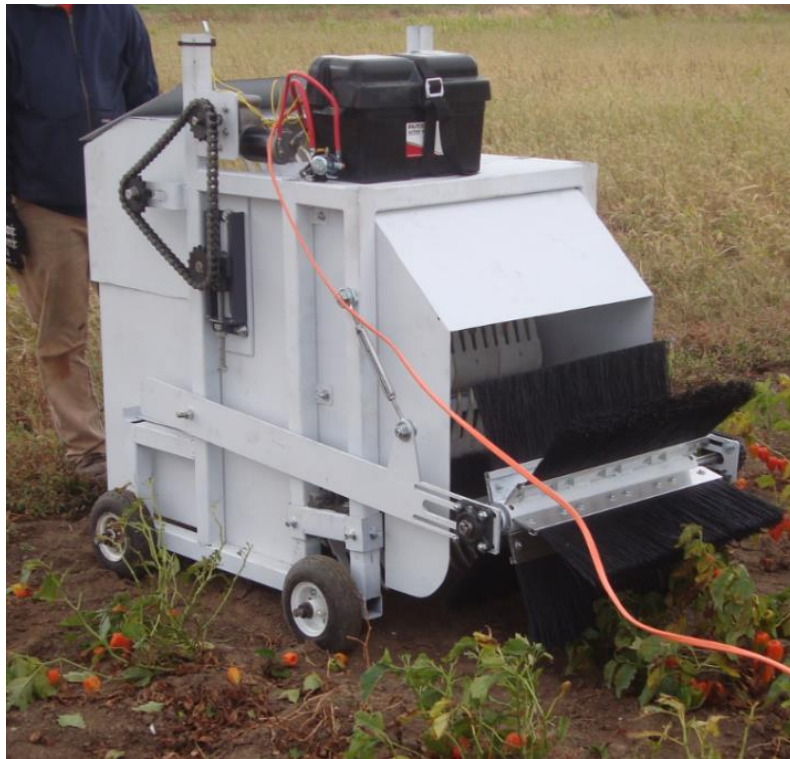
Figure 4.9: Integrated harvesting and conveyance test platform
