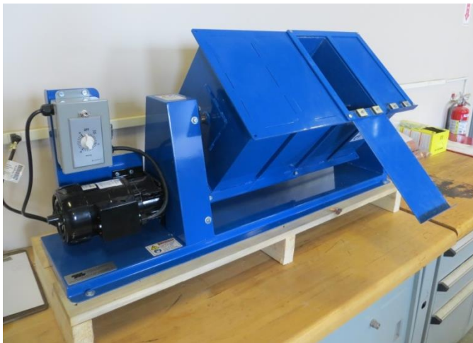
Figure 6.11: Seedburo pellet durability tester
