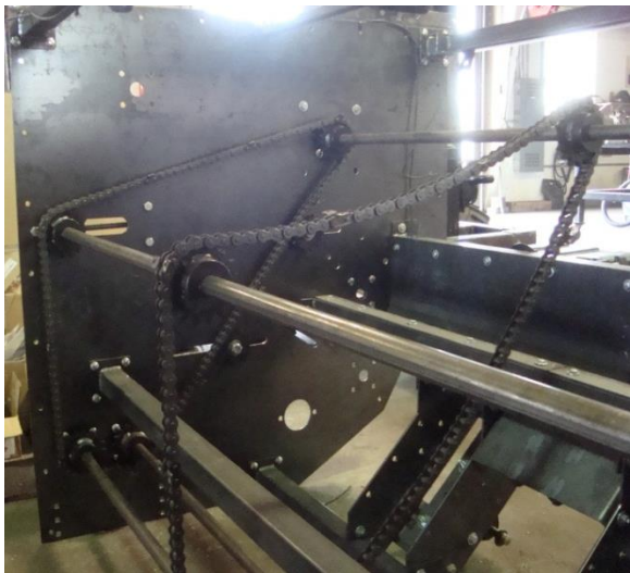
Figure 4.19: Side view of stripping header roller chain geometry
