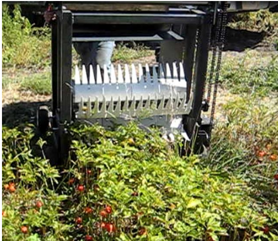
Figure 6.2: Testing of the rotary harvesting system
