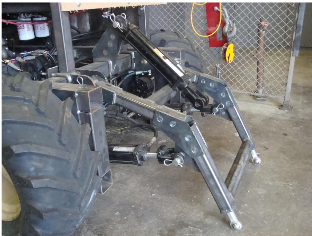
Figure 4.11: 3-Point header attachment system
