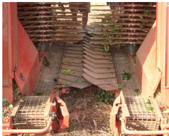
Figure 2.2: Coffee harvester catch panel floor
