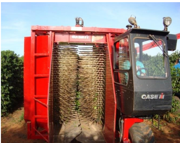
Figure 2.1: Coffee harvester with shaker columns
