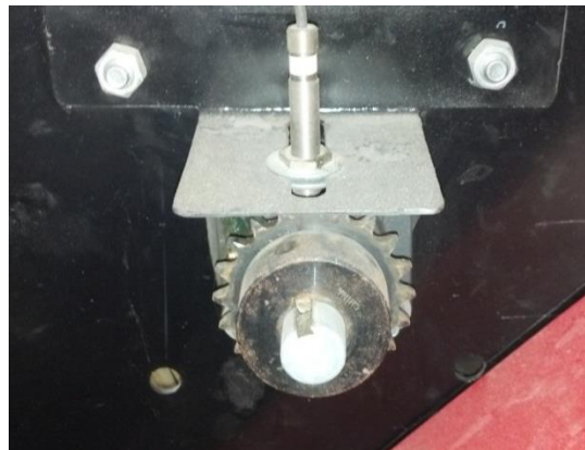
Figure 4.16: Header rotational speed sensor and sprocket
