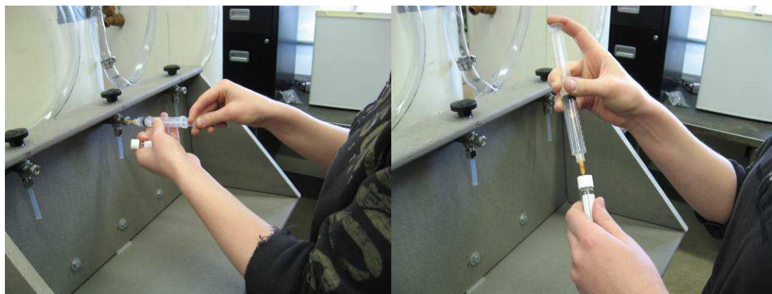
Figure 13. Pilot scale sampling station GHG collection. Left: GHG sample was collected from reactor vent line from pilot scale swine manure storage. Right: GHG sample was transferred to vial for transport to lab for analysis.
