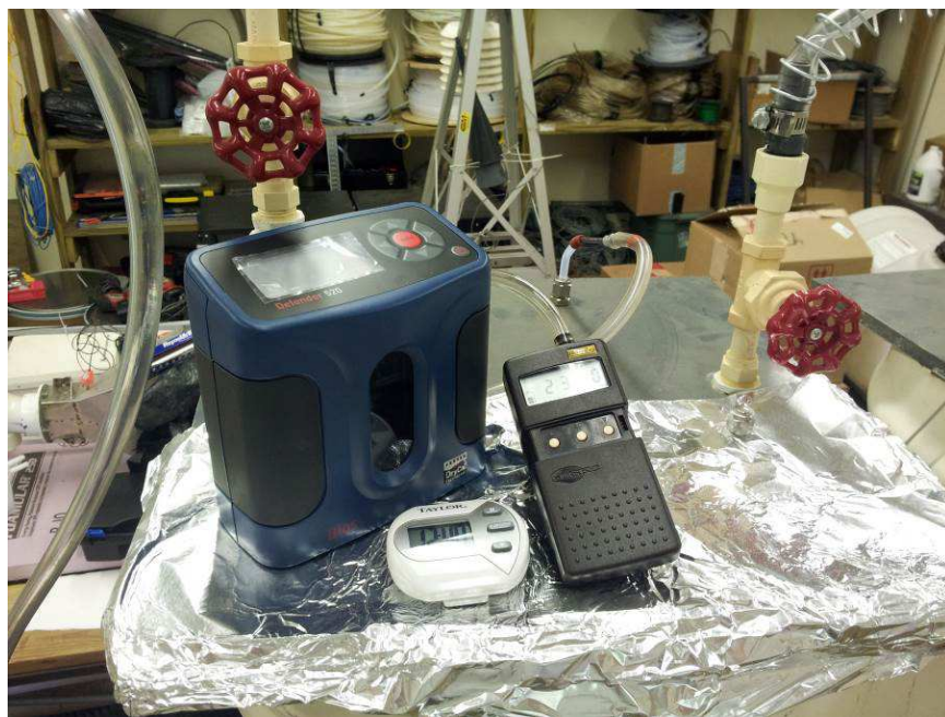
Figure 15. Pilot scale sampling setup for VOCs collection via sorbent tubes. Sampling pump pulls gas sample from the reactor vent line through the sorbent tube (4 mm O.D., 0.10 m long,
