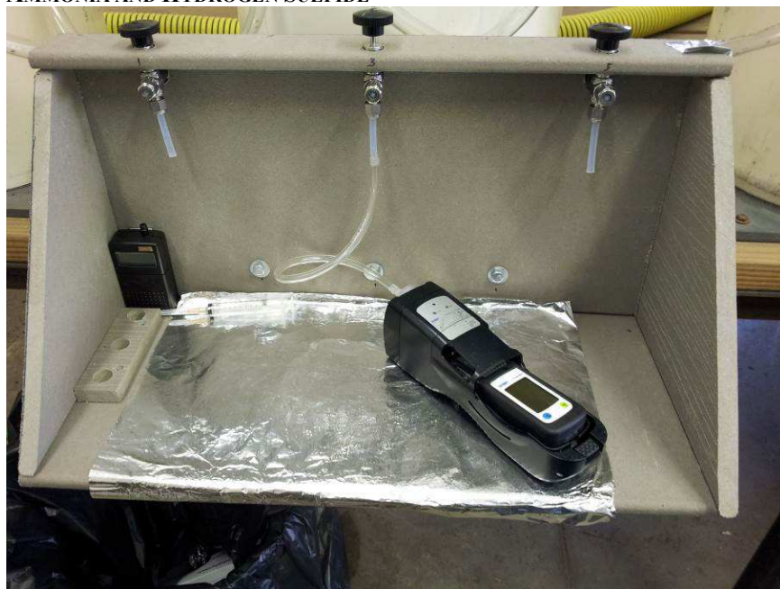
Figure 16. Drager portable gas analyzer used to measure NH_3 and H_2S from the vent line of the manure storage reactor via the gas sampling station.
