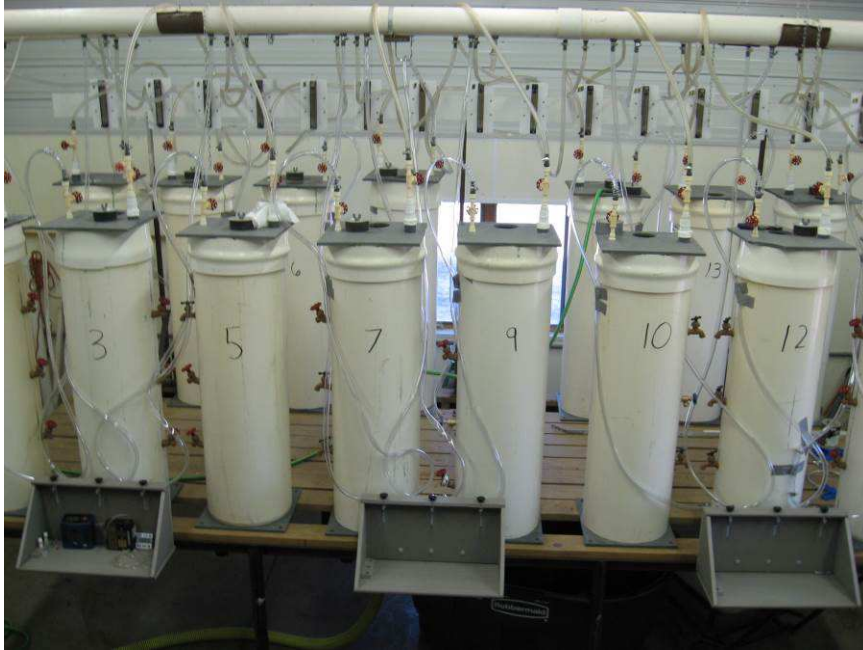
Figure 8. Pilot scale reactor setup. Fifteen 36 gal PVC reactors to hold swine manure with adjustable ventilation flow control and emission sampling stations.
