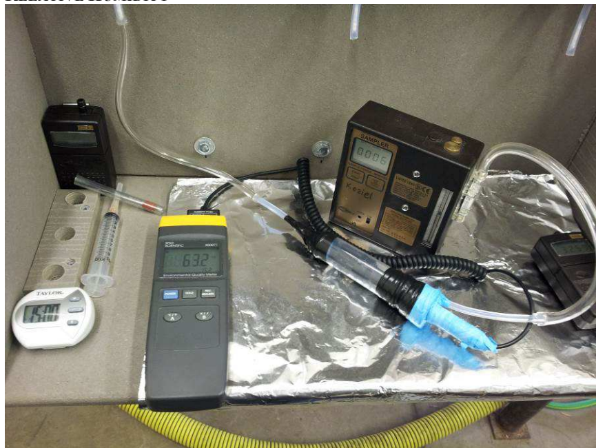
Figure 11. Pilot scale gas sampling station setup for relative humidity. Sample pump pulls air from the reactor vent line through sealed tube containing relative humidity probe.
