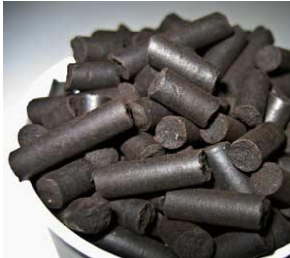
Figure 2.14: Biomass which has undergone Torrefaction Process. Source: (Google images, 2012)
