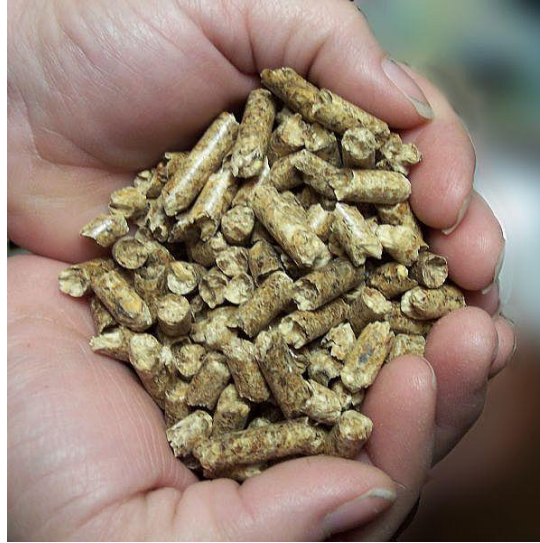
Figure 2.12: Wood Pellets Formed by Extrusion. Source: (Google images, 2012)
