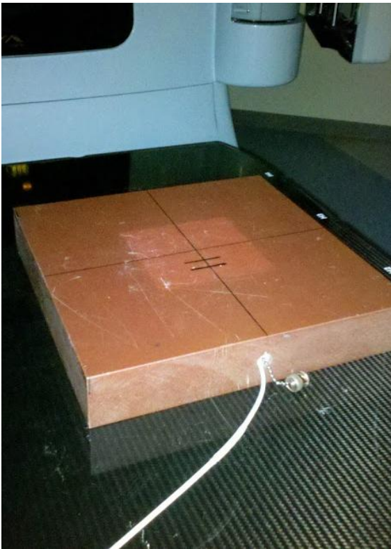
Figure 15 – Ion chamber measurement setup. Note that in this picture the triaxle cable from the control room is inserted into the solid water, thus why the cap is hanging out of it (an actual ion chamber was not placed inside for the picture, as it was not important). The light field is aligned to the center of the phantom.
