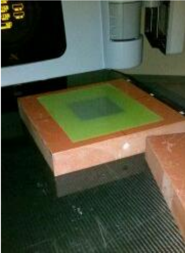
Figure 13 – Output factor measurement setup for film. The opaque square seen in the center of the film is the result of the irradiation.
