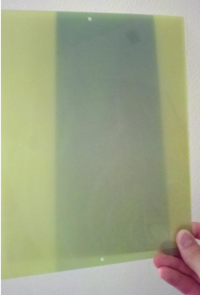
Figure 16 – The calibration film. The top of the film was the side of the film that was closest to the head of the linear accelerator, as could be deduced from the noticeable decrease in opacity from the top of the film in accordance with the inverse-square effect. Also the divergence of the beam can be noted as the image gets wider towards the bottom.
