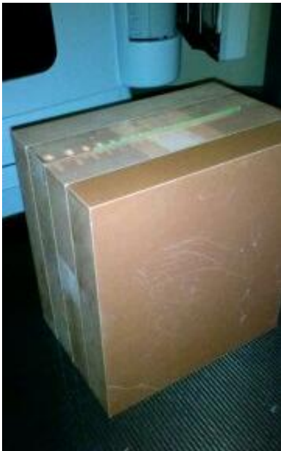
Figure 12 – Calibration setup. The top of the film can be seen sticking out between the center two solid water blocks. The light field is shown as being aligned in the center of the solid water. The treatment couch is aligned so that the top of the solid water is at 100cm SSD.
