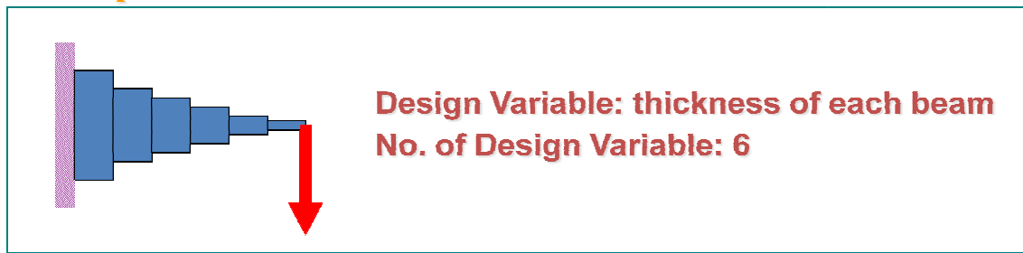
Figure 2. 4 Size optimization of beam with six elements
