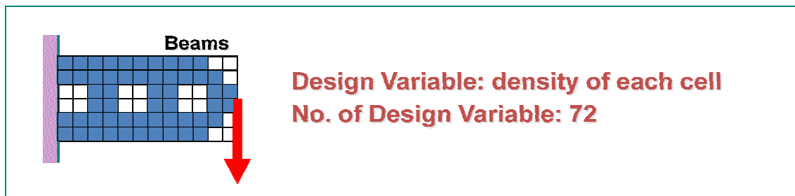
Figure 2. 6 Topology optimization of beam using density design variable
