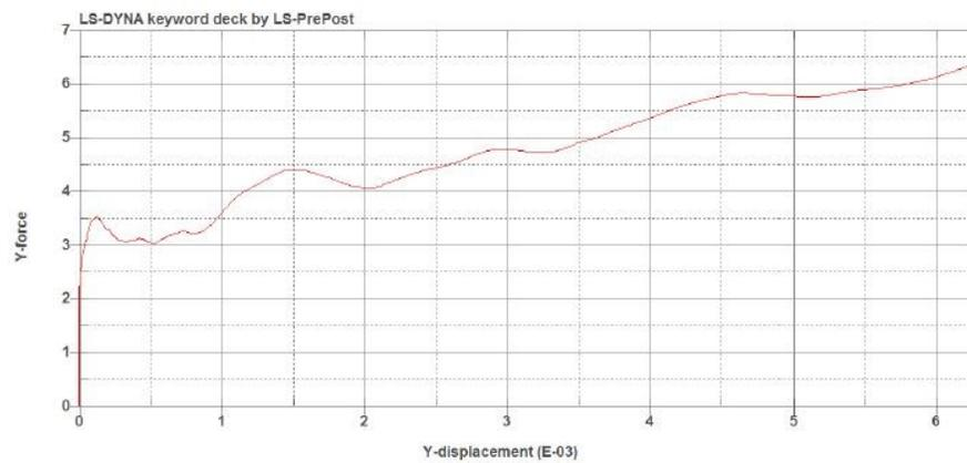
Fig. 4.2. Force-Deflection Curve. Slope=Spring constant=1.78 N/mm
