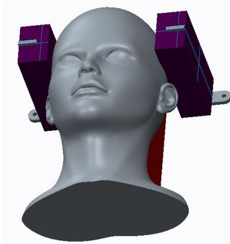
Fig. 5.12. Head Fixing Device (purple) to fix the head specially prepared in the new design
