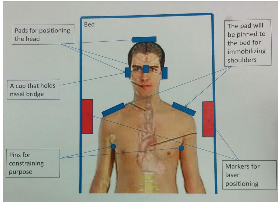
Fig. 5.10. Location of patient positioning and immobilization devices used in the new design
