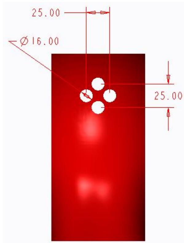
Fig. 5.27. Pressure Sensor positioning in diamond shape with dimensions
