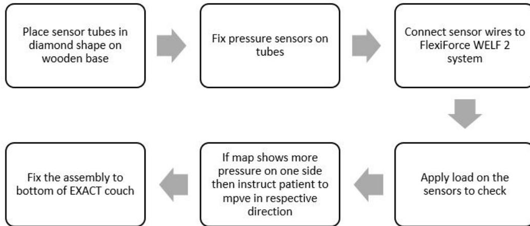
Fig. 5.29. Flowchart for preparing pressure sensor assembly
