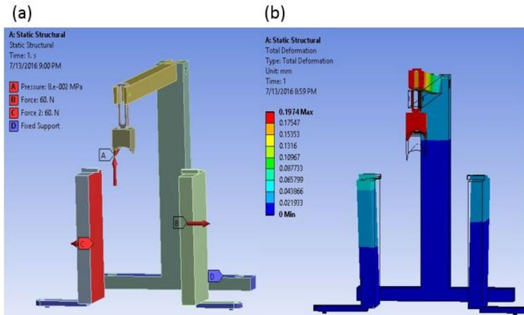
Fig. 6.3. Engineering analysis of Head fixing device (a) Input values and direction of loads, (b) Value of Deformation=0.1974 mm
