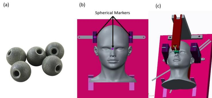
Fig. 5.4. Devices used for Tumor tracking in the new design (a) Spherical Markers, (b) Markers positioned in the new design, (c) Customized 3D printed nose bridge part (Green)
