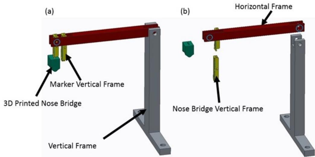
Fig. 4.1. (a) Assembly view of Stereotactic Frame, (b) Exploded View of Stereotactic Frame
