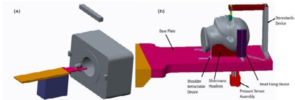
Fig. 5.5. Equipment required in the CT room for the new design (a) Complete Setup of the equipment in the CT scanning stage, (b) Description of various devices required to fix the patient rigidly in the CT scanning room
