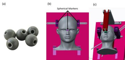
Fig. 5.13. Devices used for Tumor tracking in the new design (a) Spherical Markers, (b) Markers positioned in the new design, (c) Customized 3D printed nose bridge part(Green)
