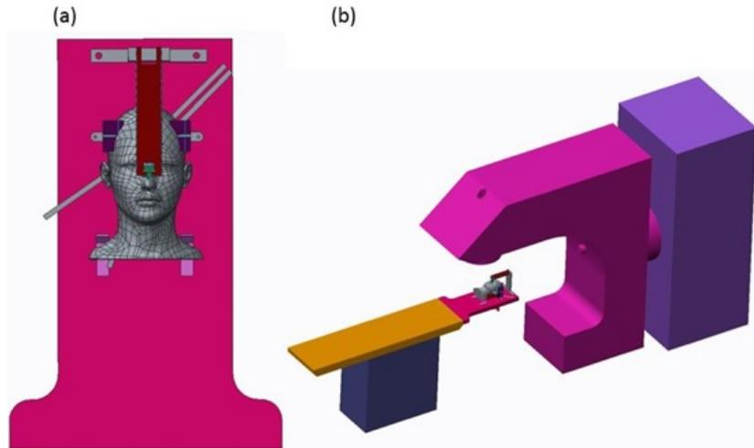
Fig. 5.24. Treatment Stage Assembly (a) Head position, (b) Overall Assembly
