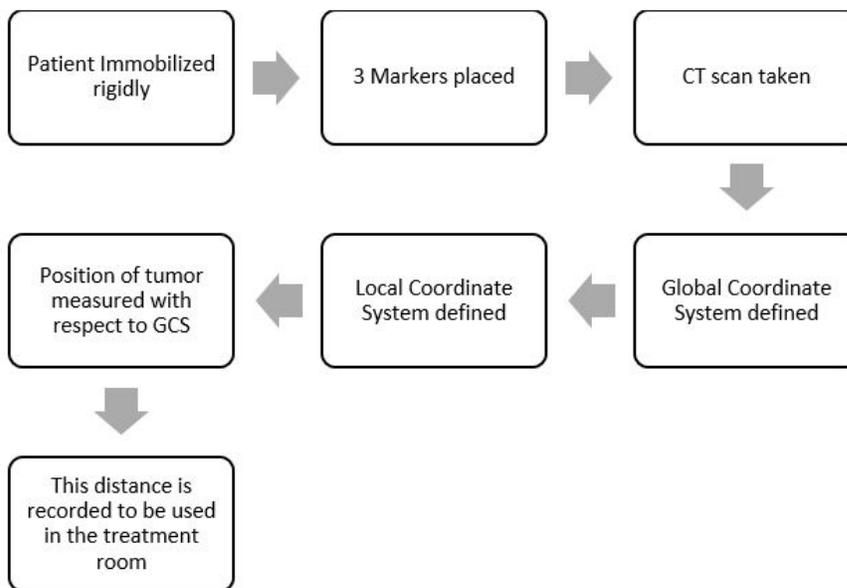
Fig. 5.17. Flowchart of tumor location in Simulation Stage
