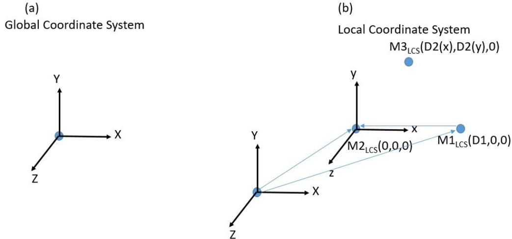
Fig. B.1. Transformation Technique with marker location in GCS and LCS
