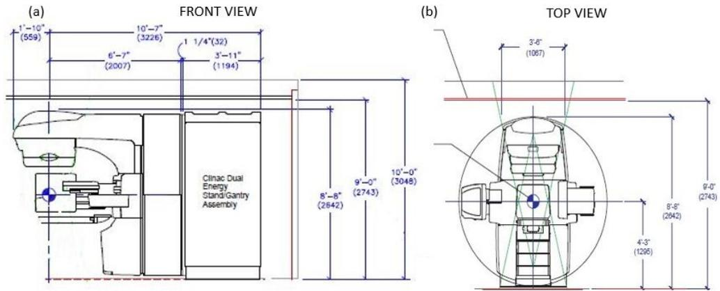
Fig. 5.7. LINAC Dimensions (a) Front View, (b) Top View
