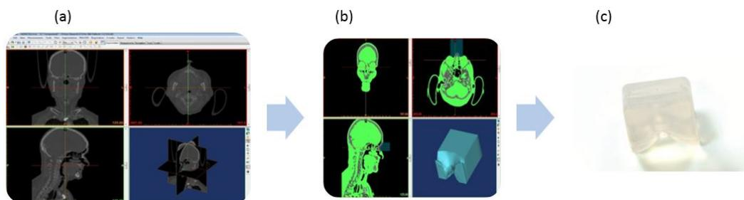
Fig. 5.30. Procedure to 3D print Nose bridge part using Materialise Mimics software (a) DICOM file of patient's CT scan, (b) 3D printed part after thresholding and cropping of 3D mask, (c) Finished product
