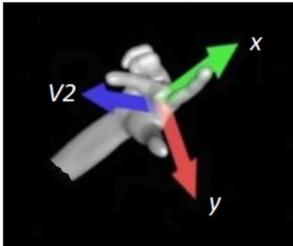
Fig. 5.18. Direction of y axis as per Right Hand Thumb Rule
