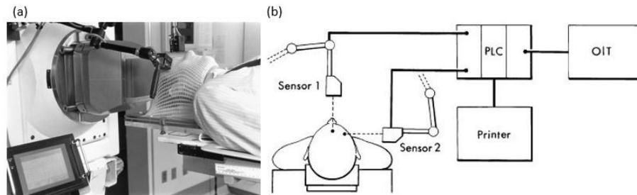
Fig. 2.1. (a) View of the patient motion monitoring system in the proton treatment room. The sensors are placed in AP and LAT direction. The OIT in the front displays the patient's motion data, (b) Schematic diagram of the patient motion monitoring system.
