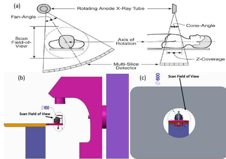
Fig. 5.3. Scan Field of View that defines the actual area of interest to scan the tumor (a) Detailed drawing, (b) SFOV (dotted line) in Treatment Room=600 mm and (c) SFOV (dotted line) in Scanning Room=600 mm
