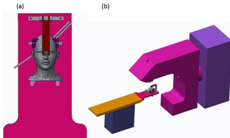
Fig. 5.8. Treatment Stage Assembly
