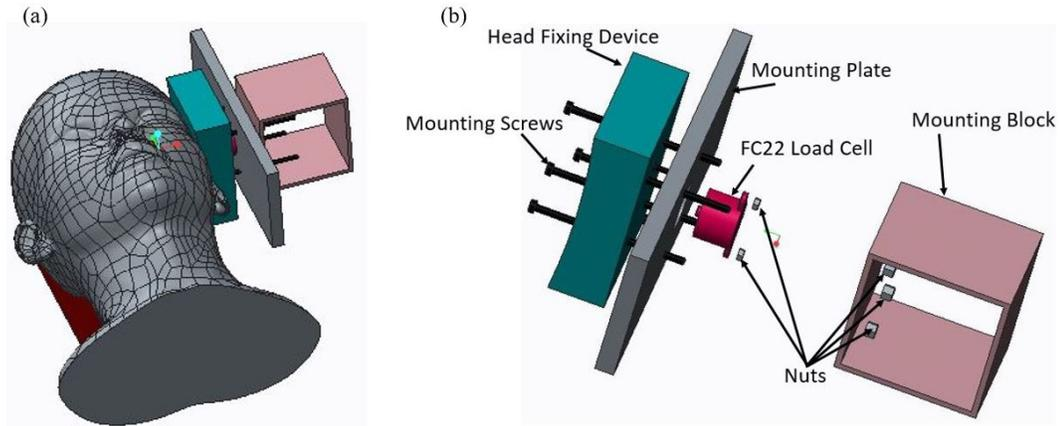
Fig. 6.1. Experimental setup to calculate amount of load patient exerts on the immobilization devices for doing the analysis on ANSYS software (a) Experimental Setup with 3D printed part touching patients face for load calculation and (b) Exploded view of the assembly
