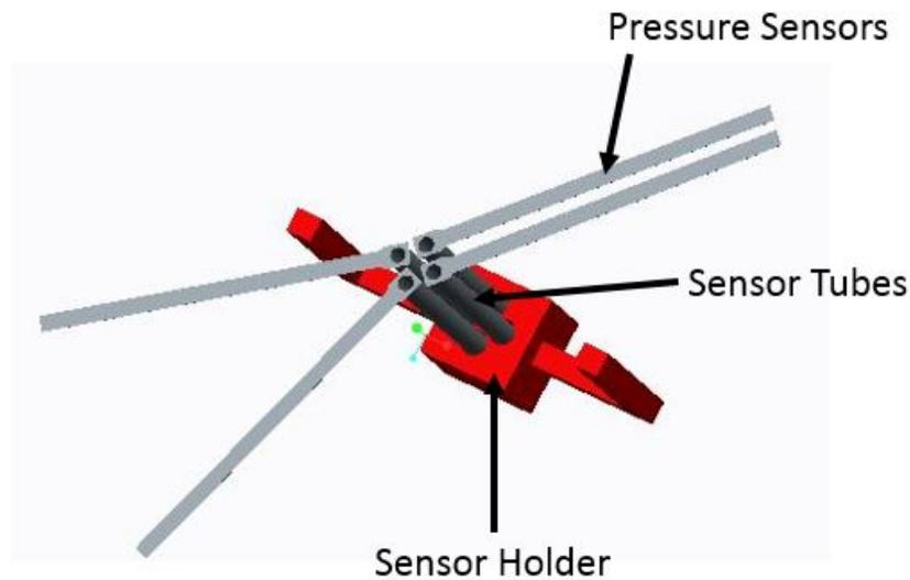
Fig. 5.26. Pressure Sensor Assembly
