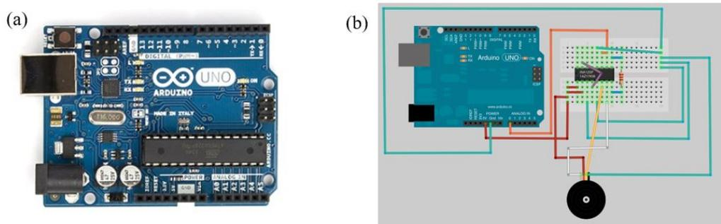
Fig. 6.2. Arduino Uno kit used to generate the code for load calculation (a) Arduino Uno circuit board (*CourtesyofArduino*<sup>®</sup>), (b) Arduino Uno breadboard connections[40]
