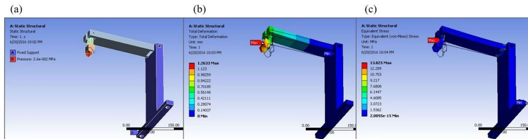
Fig. 6.4. Engineering Analysis of Stereotactic Device (a) Fixed support and Pressure location, (b) Deformation=1.2633 mm and (c) Stress=13.825 MPa
