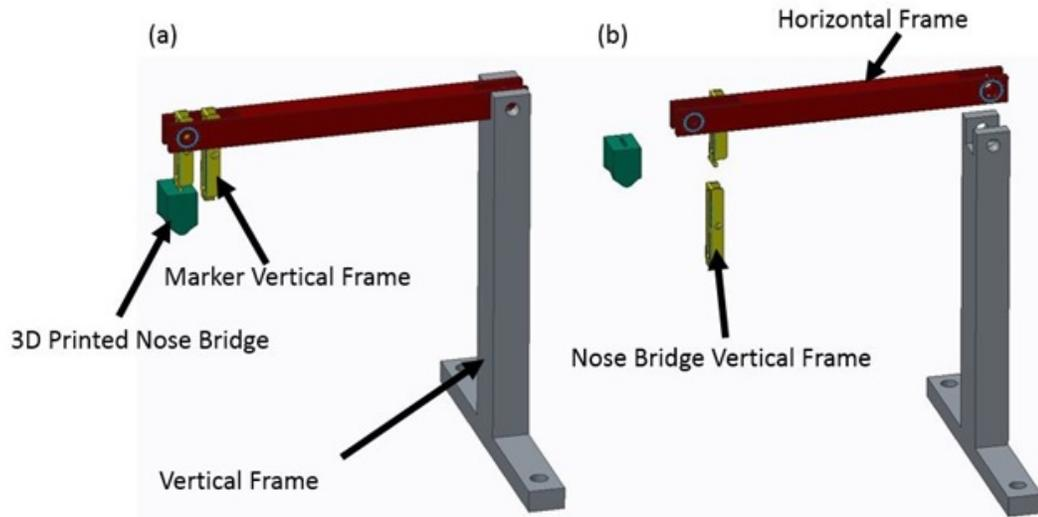
Fig. 5.31. (a) Assembly view of Stereotactic Frame, (b) Exploded View of Stereotactic Frame
