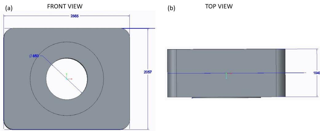
Fig. 5.6. CT Machine dimensions (a) Front View, (b) Top View
