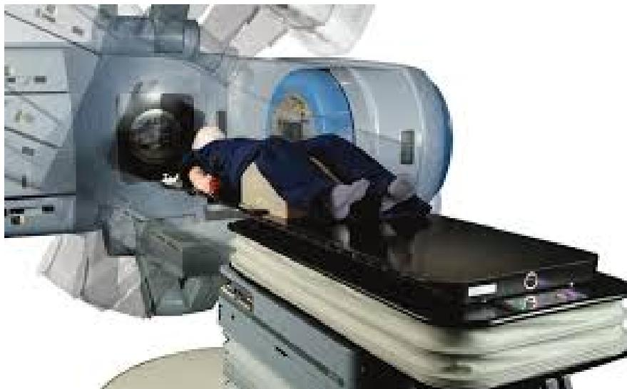
Fig. 1.3. Linear Accelerator (LINAC) Treatment Machine used in VAMC, Indianapolis, Indiana, USA to treat the cancerous tumor cells (Courtesy of Varian Medical Systems Inc.<sup>TM</sup>)
