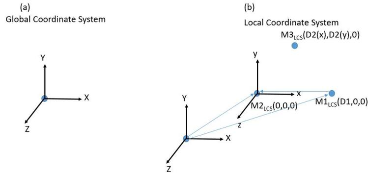
Fig. 5.16. Coordinate Transformation (a) Global Coordinate System (GCS) with coordinate axes X, Y and Z, (b) Local Coordinate System (LCS) with coordinate axes x, y, z and location of new markers M1, M2 and M3 with respect to GCS
