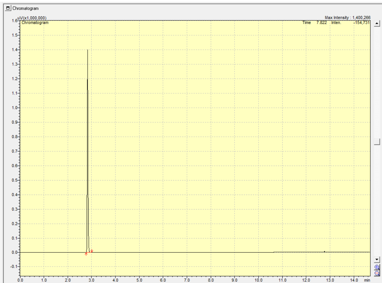
Figure 8: 1% EtOH Standard Chromatogram
