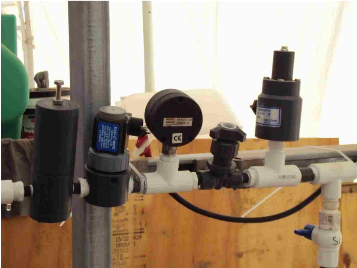
Figure 54: Control Sequence at Pilot Input including Pressure Reducer, Solenoid Valve, Pressure Gauge, Needle Valve, and Pressure Relief Valve
