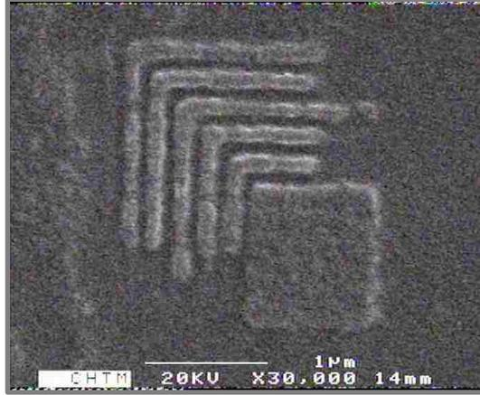
Fig. 3.42 SEM of developed PR for 3-exposure IIL for a  $CD$  of 100-nm ( $k_1 = 0.37$ ) at a 244-nm wavelength and 0.9  $NA$ . Isolated lines and the square edge of the box are well defined; dense lines are cleared.
