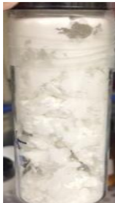
Figure 6. The synthesized gallium precursor, [(\text{CH}_3)_2\text{NH}_2]\cdot\text{GaCl}_4 .
