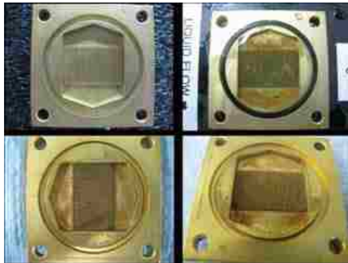
Figure 6.8 Results for corrosion testing of gold plated samples are shown. The top left picture is before testing, the others are post testing.
