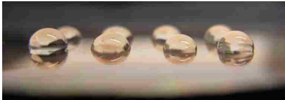
Figure 5.1 Droplets were placed at multiple locations on the vapor chamber lid to test for hydrophobicity.
