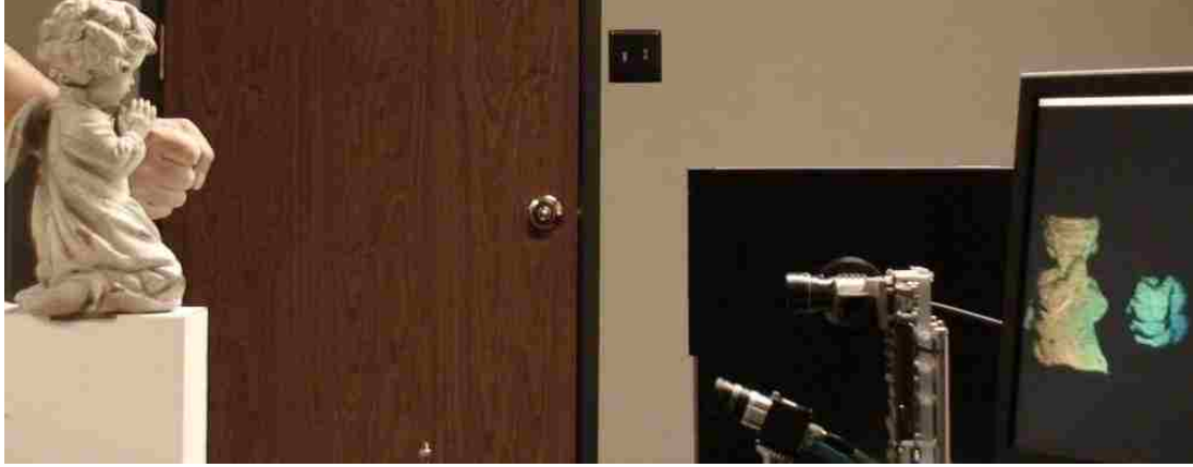
Figure 3.14: Realtime 3-D reconstruction employing proposed PCPS strategy. The frame rate achieves 120 fps.
