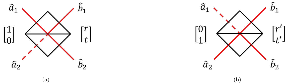
FIGURE 4.1. Representation of beam splitter transformation. The annihilation operators transform from \hat{a} to \hat{b} . Figure (a) shows a source incident on the top mode of the beam splitter and transforms the jones vector in unprimed notation, while figure (b) illustrates incidence from the bottom and transforms to primed notation. Here, r and t are completely general coefficients.
