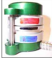
1. To disassemble the CPEM, remove the screws and green top.
