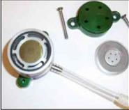
3. To insert/remove a 25mm Teflon filter into the Red stage, first use the C-clamp pliers to remove the C-ring under the Red stage (be careful that it doesn't fling off).
