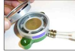
5. Insert a 25mm Teflon filter into the Blue stage following the instructions in step 3. Again, note the "B" on the plate for "bottom".
