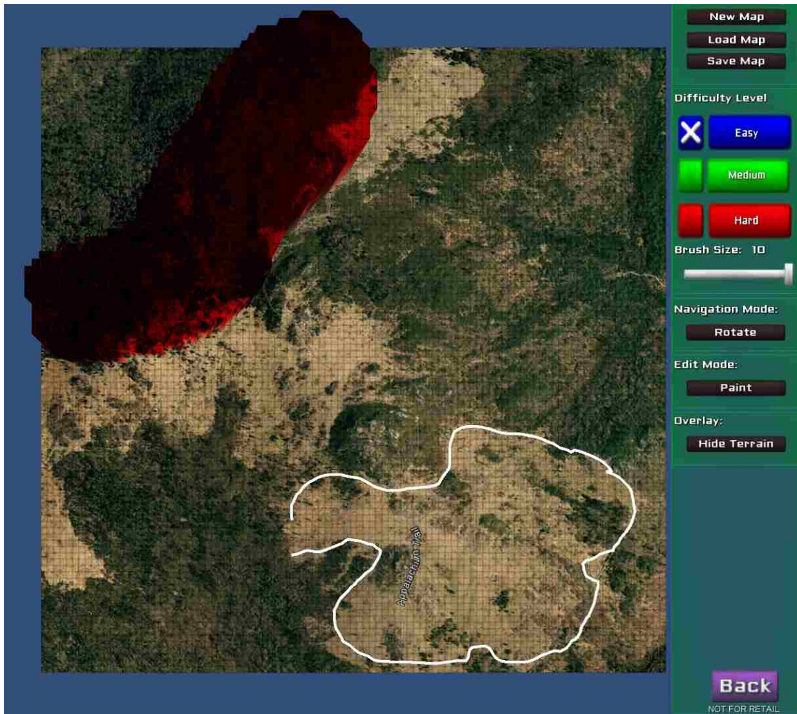
Figure 7.4: A satellite imagery of the search area loaded into the DiffEdit tool as an overlay, an example high task-difficulty area on the top left corner made using the paintbrush tool, and an example selection made using the lasso selection tool.
