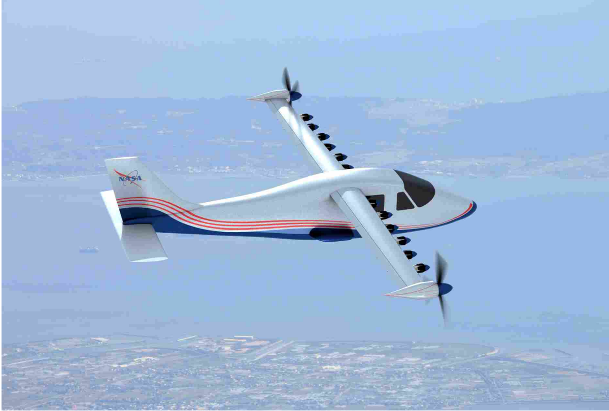
Figure 1.1: Illustration of the NASA X-57 thin-haul concept aircraft showing the mid span DEP propellers in the folded cruise position. (Image reprinted from “NASA Electric Research Plane Gets X Number, New Name”, by A. Beutel, 2017, Retrieved from https://www.nasa.gov/press-release/nasa-electric-research-plane-gets-x-number-new-name . Public Domain Credit: NASA)
