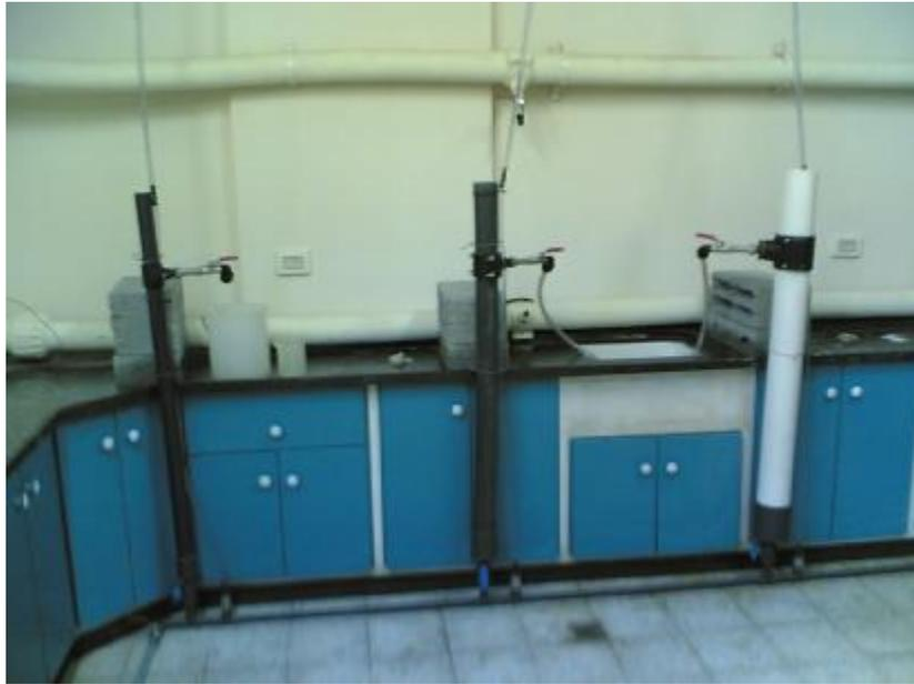
**Figure D. 1 Up-flow Reactors were used**
