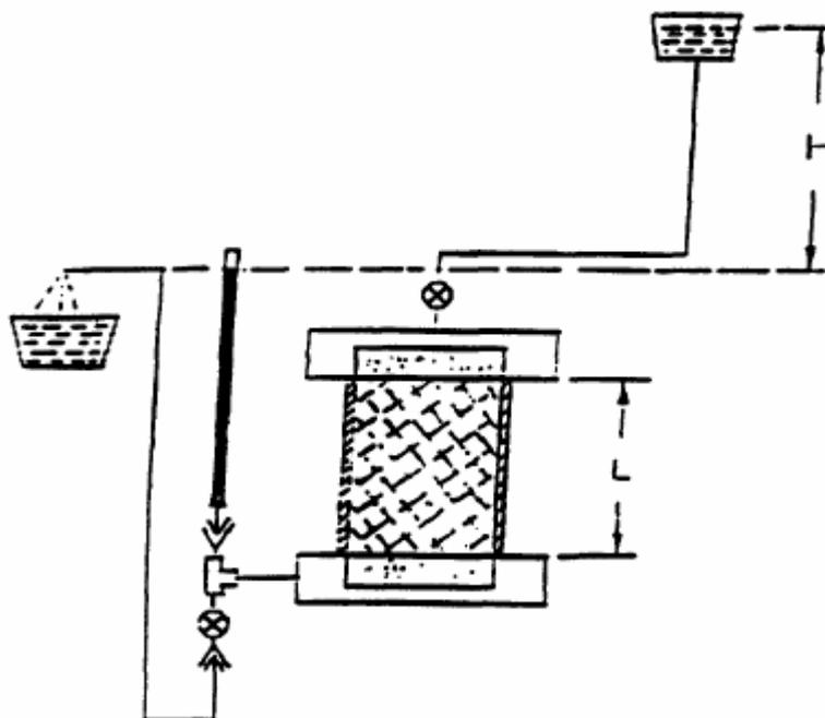
Figure3. 2 Constant head permeability test
