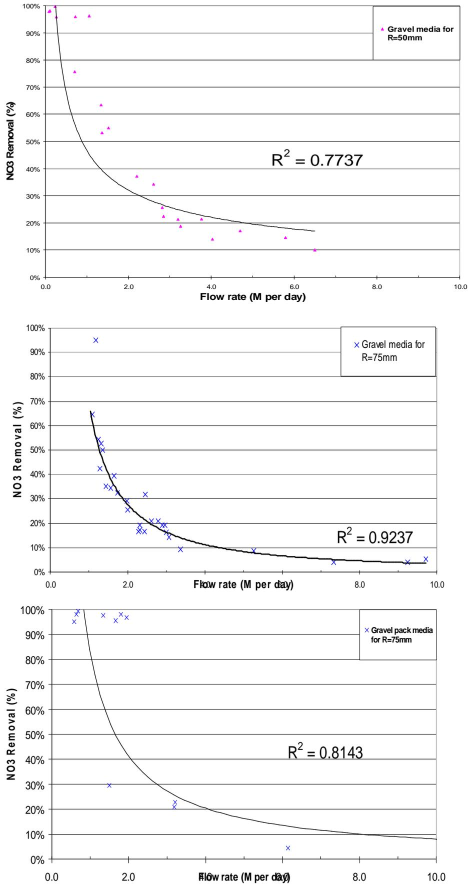
Figure4. 5 Relationship between nitrate removal and flow rate velocity
