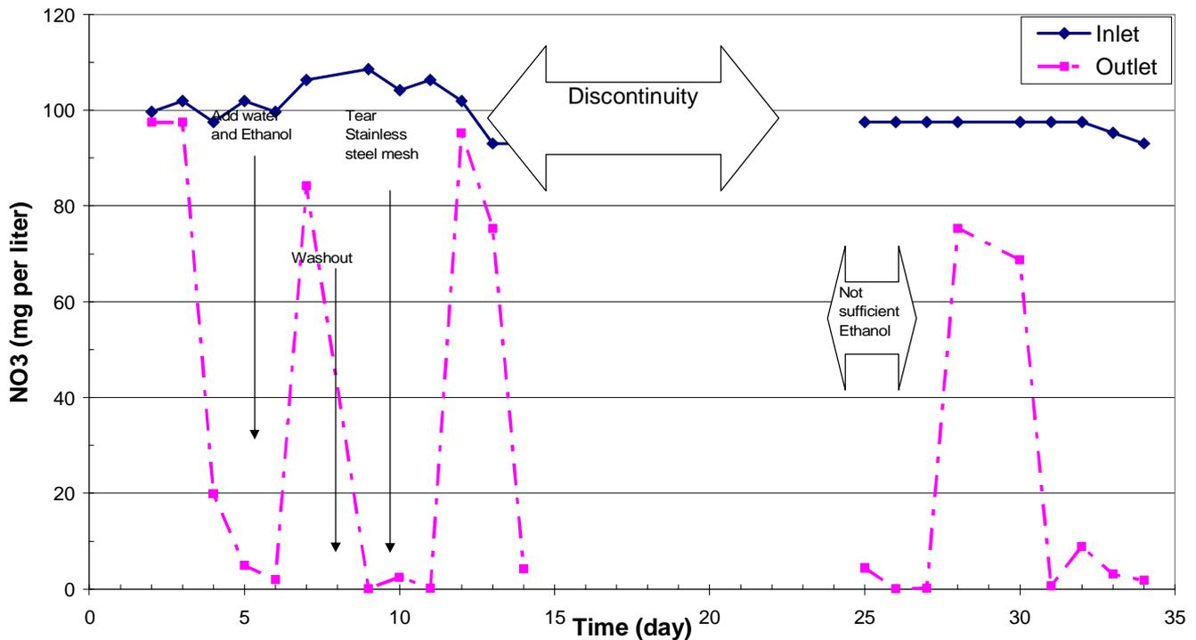
**Figure4. 4 Time course of nitrate removal in gravel pack column reactor d=75 mm during the operational period (35 d).**
