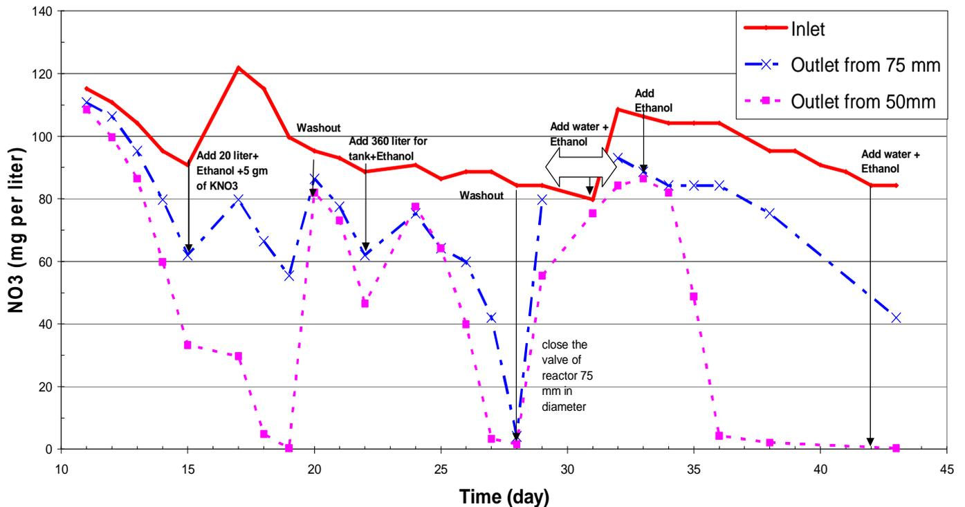
**Figure4. 3 Time course of nitrate removal in Gravel column reactor d=50mm and d=75 mm during the operational period (43 d).**
