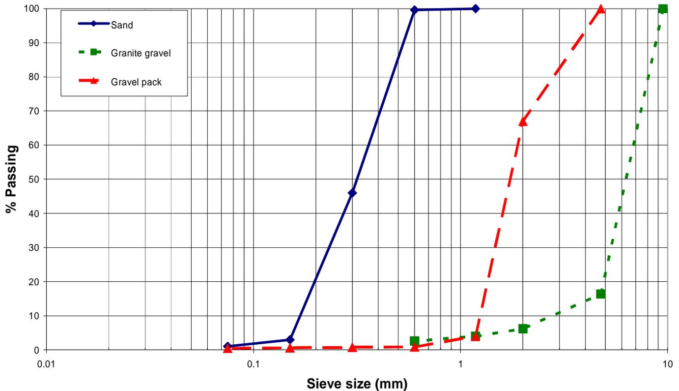
Figure4. 1 Grain size distribution of filter materials
