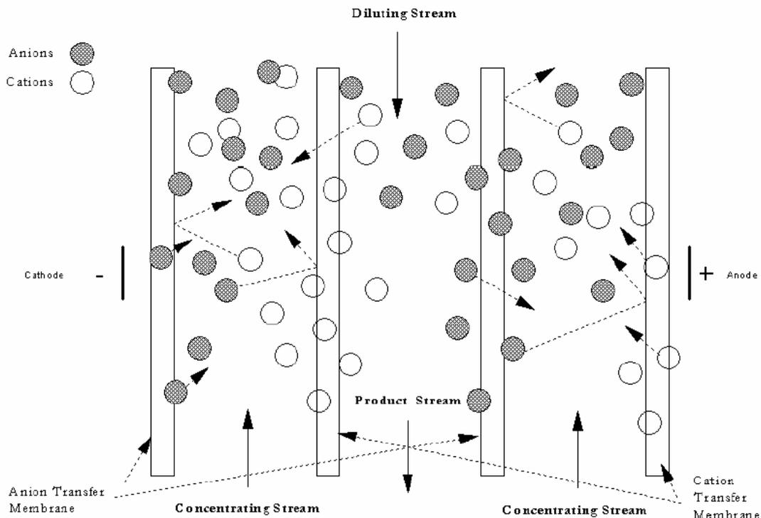
**Figure 2.3** Transfer of ions within the electrodesalination stack
