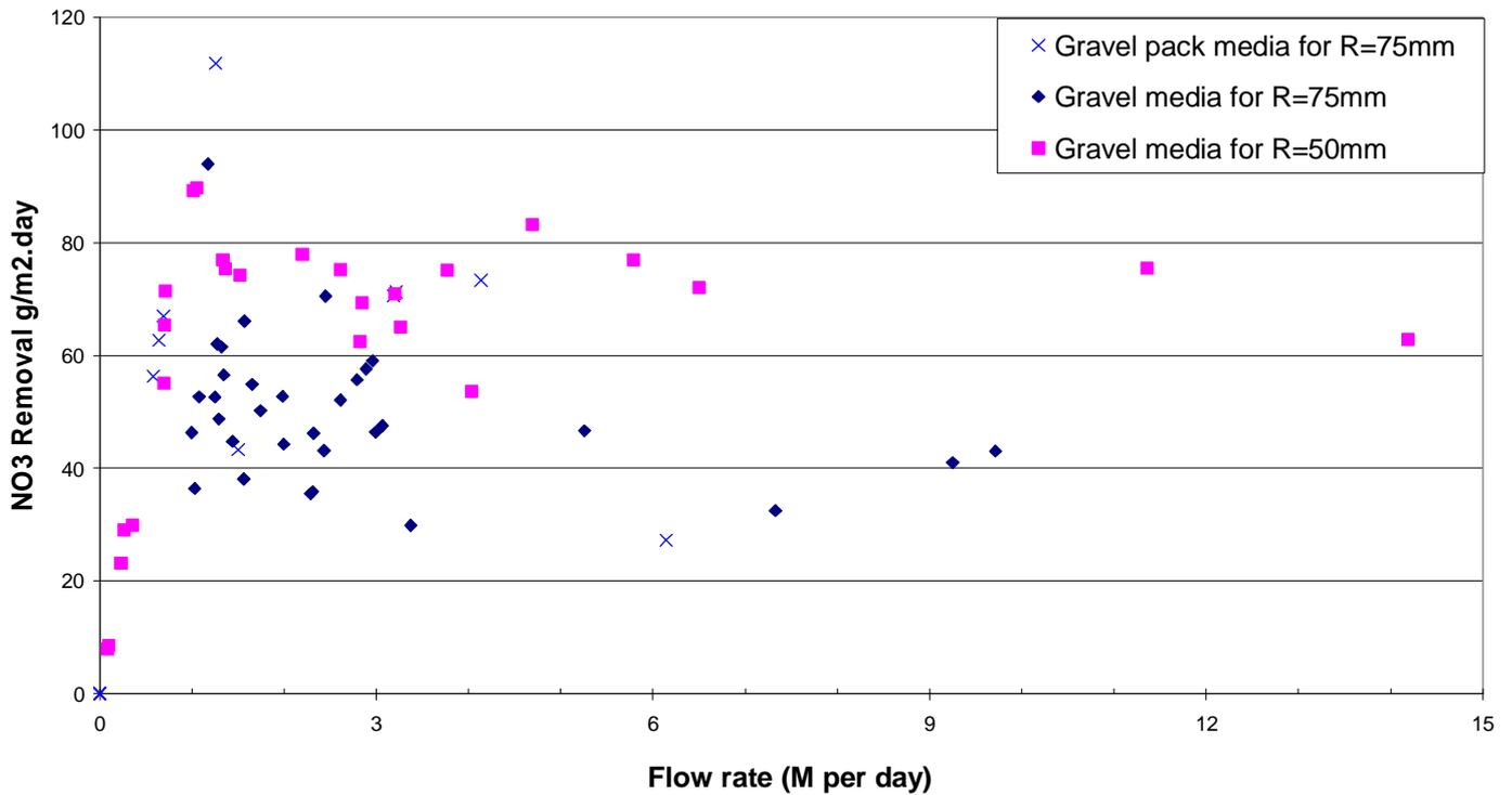
**Figure 4. 6 Relationship between surface load removal  $\text{mg}\cdot\text{m}^{-2}\cdot\text{day}^{-1}$  and flow rate velocity**
