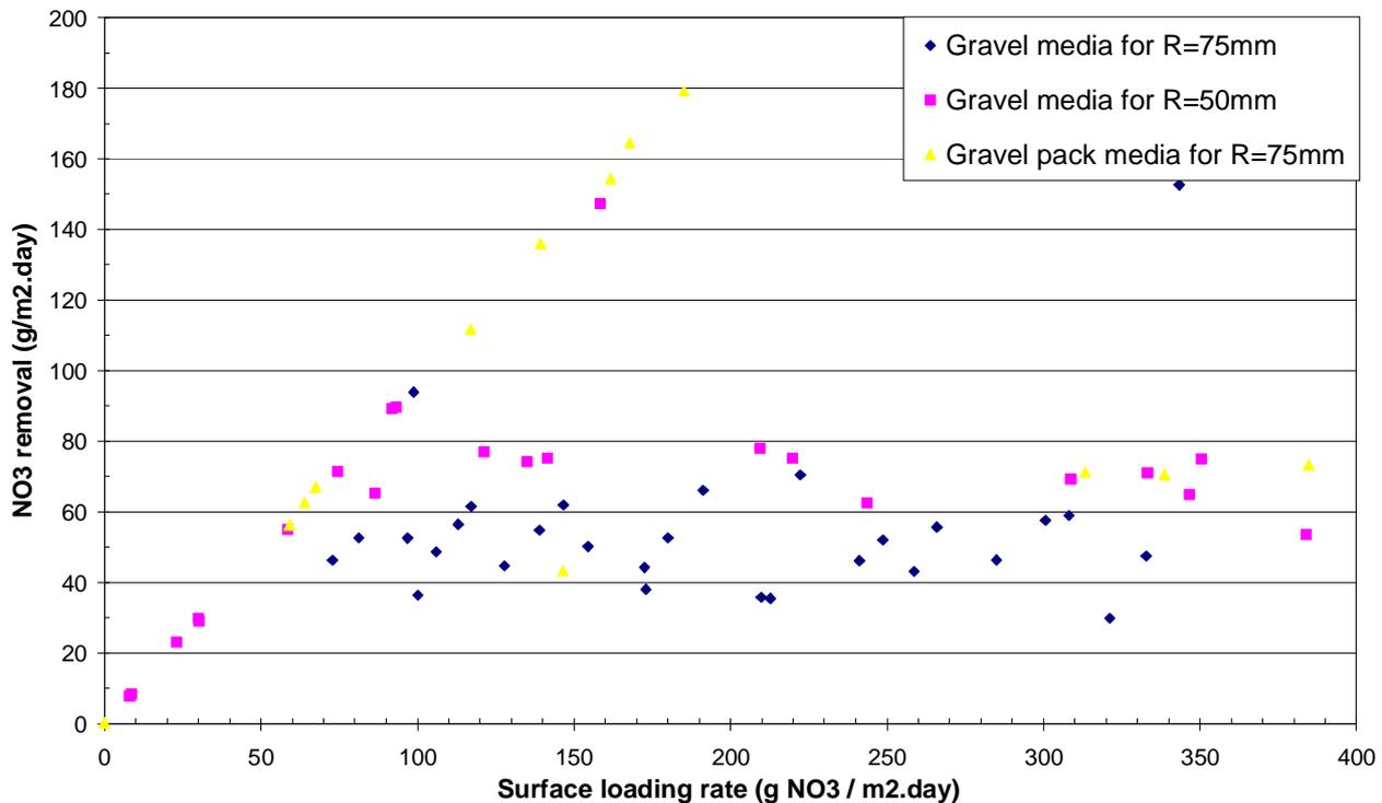
**Figure 4.7 Relationship among surface loading rate  $\text{g}\cdot\text{m}^{-2}\cdot\text{d}^{-1}$  inlet and outlet**
