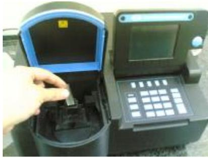
**Figure D. 8 Spectrophotometer (Hach DR 4000U UV) was used to measure nitrate**
