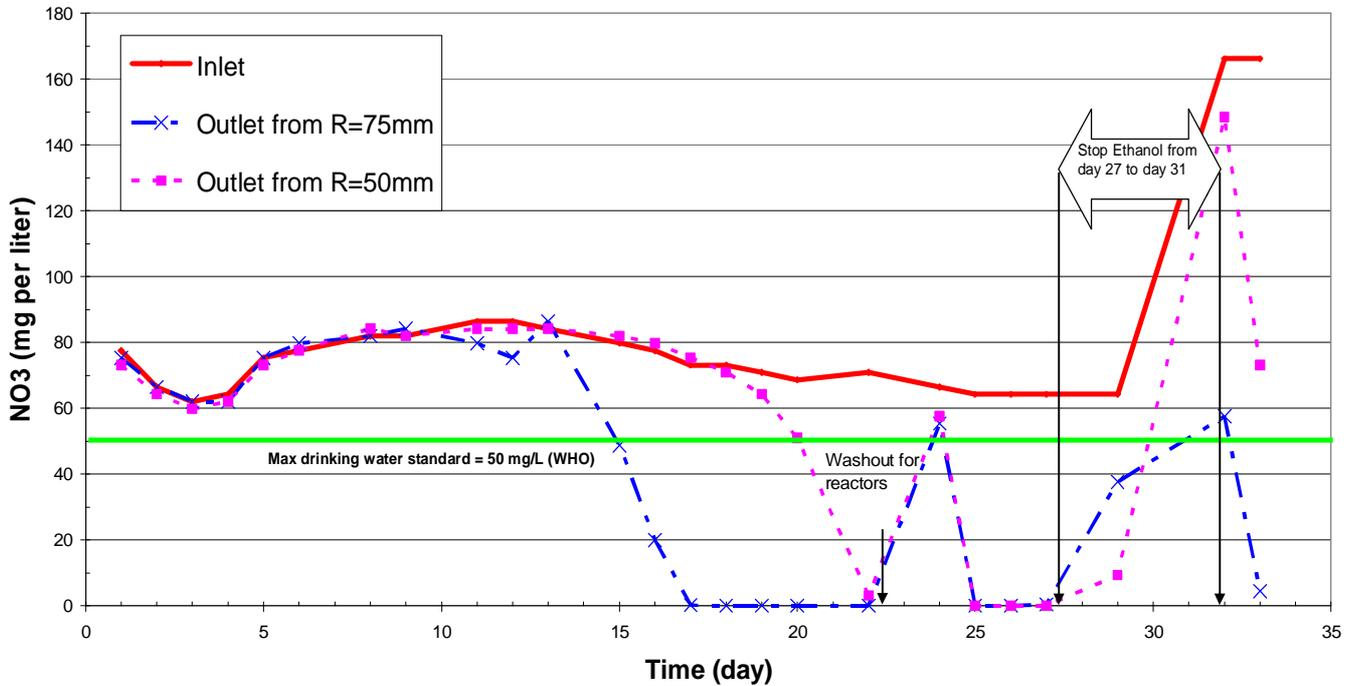
**Figure4. 2 Time course of nitrate removal in sand column reactor d=50mm and d=75 mm during the operational period (33 d).**
