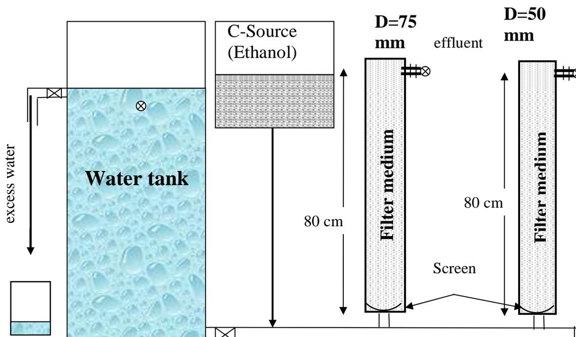
Figure3. 1 Schematic diagram of the system
