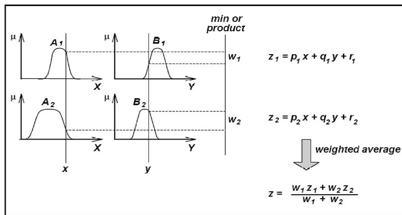
Figure (3.9): Fuzzy Inference Processing using TSK Model
