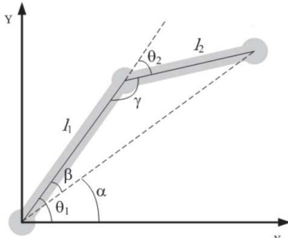
**Figure (A.1):** Geometric of two revolute links of the manipulator
