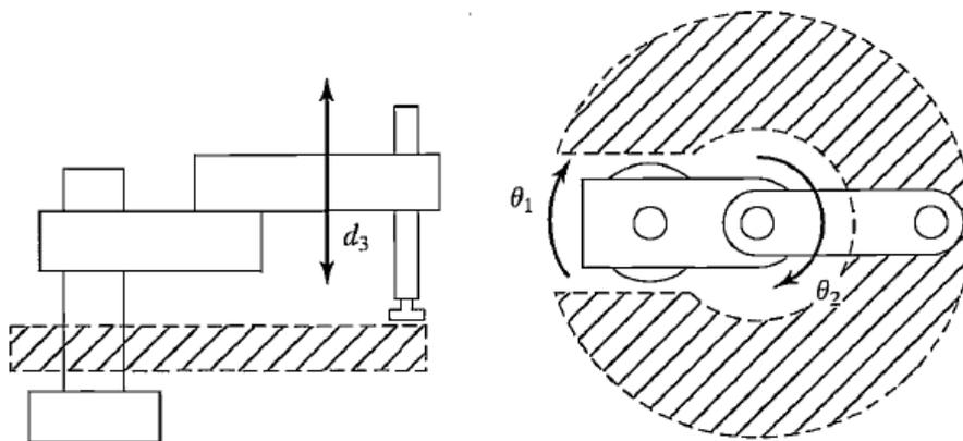
*Figure (3.11): Side view and Top view for 3-link Manipulator*
