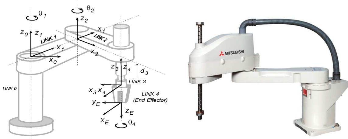
*Figure (3.12): Three-link SCARA Manipulator*
