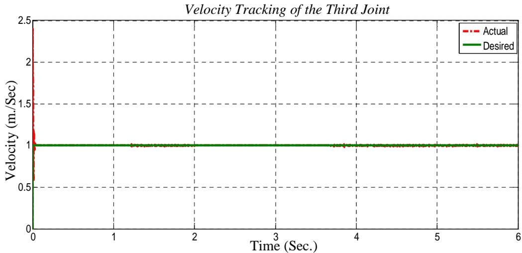
**Figure (4.14):** Velocity Tracking Curve of the Third Joint
