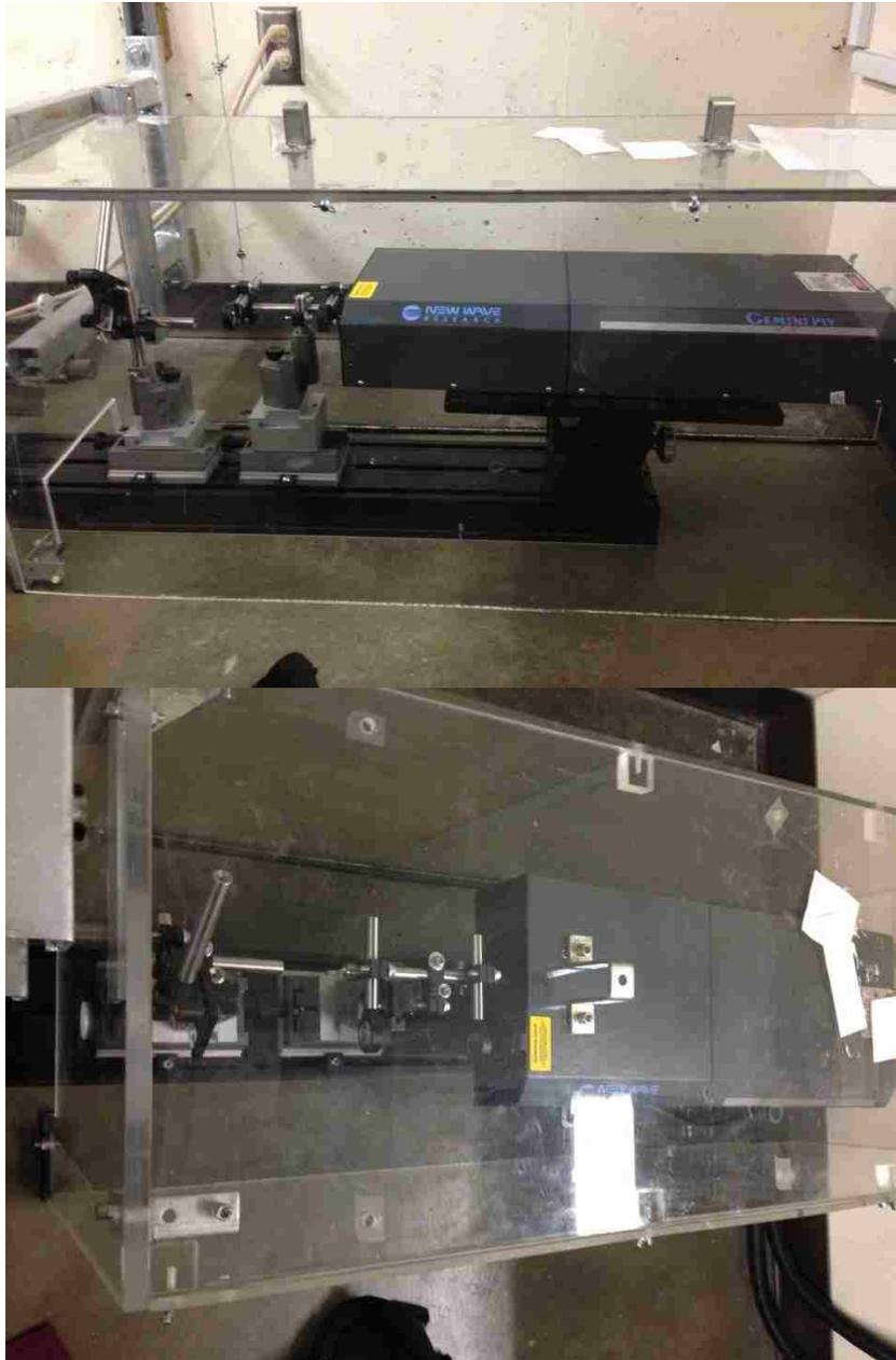
Figure3.3.1: Right and top views of Laser and lens system. The system is housed in a Lexan enclosure to protect the lenses from dust, accidental damage and shock wave effects during experimental runs.
