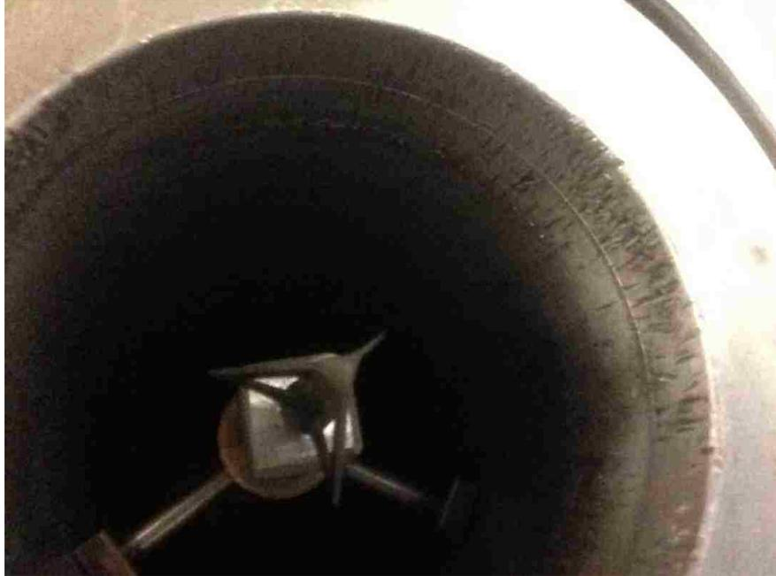
Figure 3.1.3: Solenoid driven puncture head in the driver section housing.
