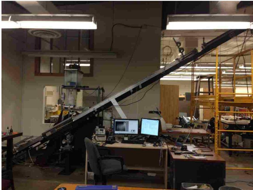
Figure 3.1.2.: Photograph of the overall shock tube laboratory setup (tilted at a 30 degree angle to the horizontal). The control center (pictured in the middle) is where the data collection occurs.
