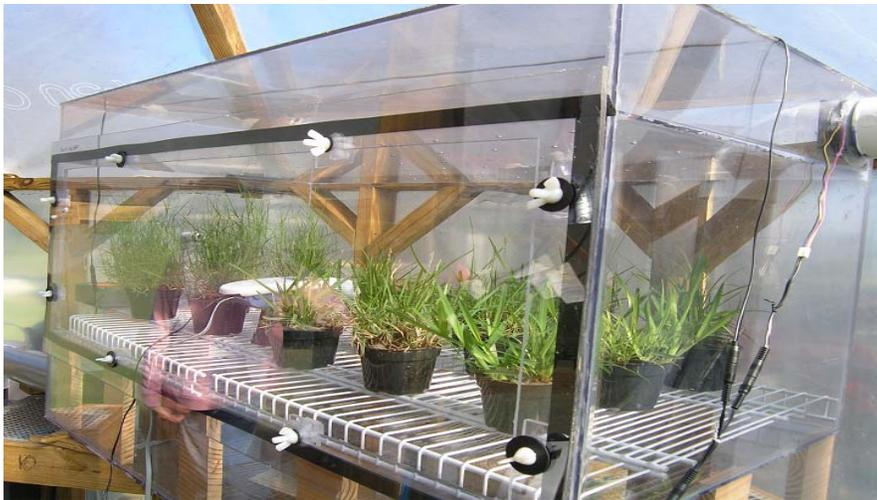
Figure 2.2. Fumigation chamber designed for 2007 and 2008 ozone studies.
