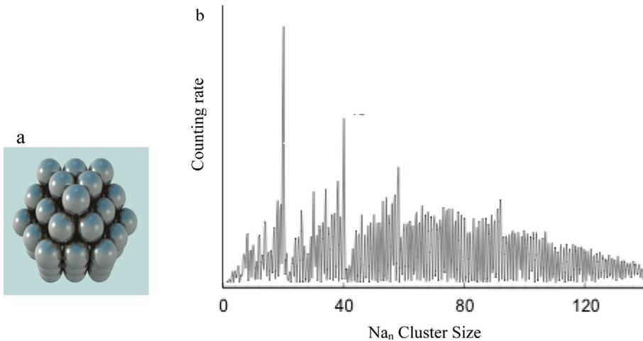
**Fig. 1.** (a) Cluster; (b) abundance in mass spectra. Vertical axis: number of electrons per cluster (counting; the peaks in stability correspond to “magic” clusters).
