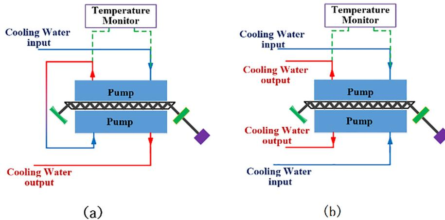
**Fig. 4.** Experiment setups with cooling water (a) series and (b) parallel connected (blue line indicate the LDAs cooling water input and red line indicates output). Two cavity mirrors were used to test the energy storage of the module. (For interpretation of the references to colour in this figure legend, the reader is referred to the web version of this article.)
