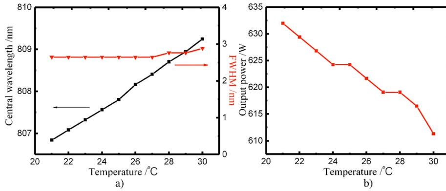
Fig. 2. Temperature property of LDAs, a) output spectrum peak wavelength and FWHM and b) output power as function of temperature under the same pump current.
