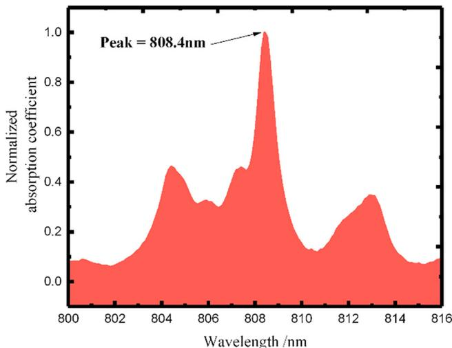
Fig. 1. An typical absorption spectrum (normalized) of Nd:YAG. The absorption peak was at 808.4 nm.
