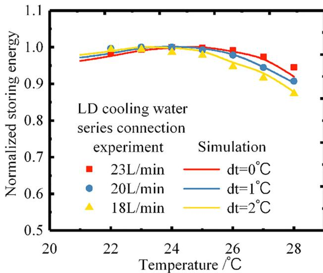
**Fig. 5.** The experiment and simulation energy storing results (normalized), under the condition that cooling water pipes were in series connected and pump current was 120 A.
