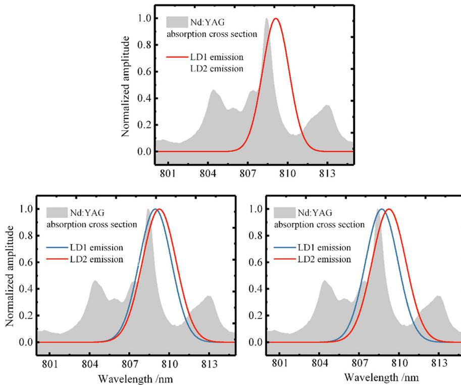
Fig. 3. The spectrum overlap between Nd:YAG absorption spectrum (gray shadow) and LDAs emission spectrum (colored line). (For interpretation of the references to colour in this figure legend, the reader is referred to the web version of this article.)
